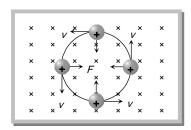
$\theta = 90^{\circ}$ , hence from  $F = qvB \sin\theta$  particle will experience a maximum magnetic force  $F_{max} = qvB$  which act's in a direction perpendicular to the motion of charged particle. (By Flemings left hand rule).
