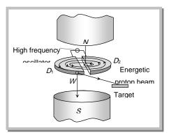
It consists of two hollow D-shaped metallic chambers  $D_1$  and  $D_2$  called dees. The two dees are placed horizontally with a small gap separating them. The dees are connected to the source of high frequency electric
