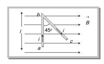
Solution: (c) Force on portion ab of wire  $F_1 = Bil \sin 90^\circ = Bil$
